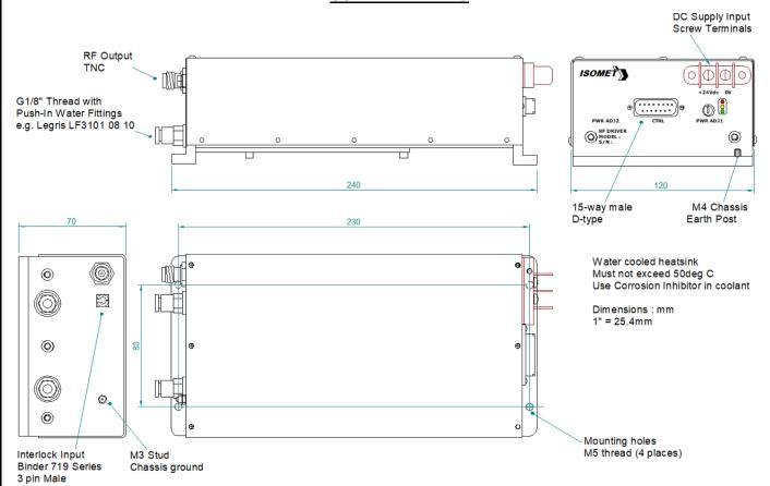
Heatsink in contact with coolant water. Default aluminium. See BR option. Water-coolant fittings supplied are suitable for 8mm OD / 6mm ID pipe.
